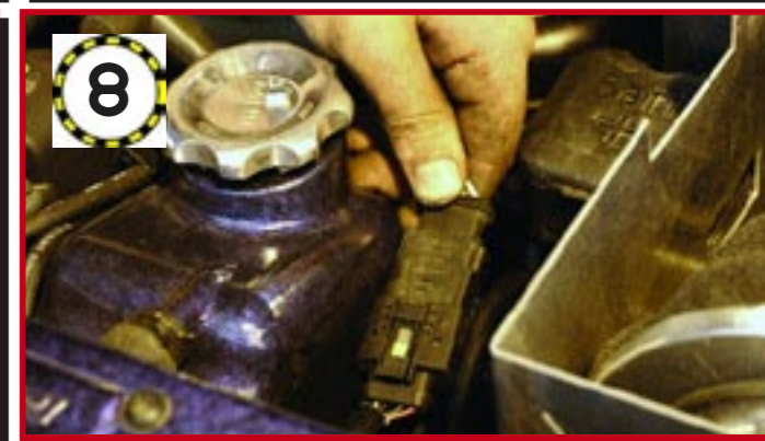
8 Remove the jack and stand. If you intend to remove the exhaust manifold, lift the bonnet and unclip the lambda sensor plug, which is connected to the side of the cylinder head, just below the oil filler cap
