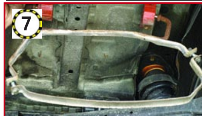
7 If the exhaust you're fitting doesn't need the standard clamp for the rear silencer, it can be removed completely. It is fitted with four 13mm nuts into the underneath of the floor
