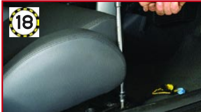
18 Slide the seat fully back, then fit the front Torx T30 bolts for the runners. The runners and seat may need to be moved to locate the bolts, so make sure the rear bolts are loose
