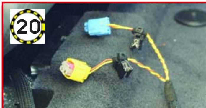
20 Reconnect the airbag (if fitted to the new seat) and seatbelt tensioner wires. Switch on the ignition and check that no warning lights appear
