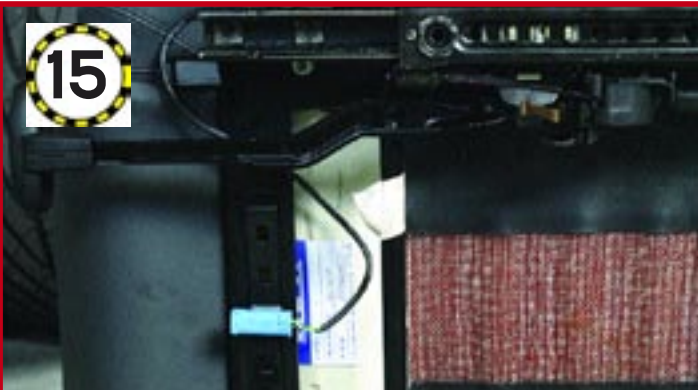
15 Feed the wire for the seat belt tensioner under the seat and clip the connecting plug in place. Use plastic ties to secure the wire and make sure it doesn't obstruct the runners
