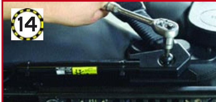
14 Refit the seat belt unit and tensioner, which was removed in step 9. Fully tighten the Torx T45 bolt. Make sure the wire for the tensioner is not trapped
