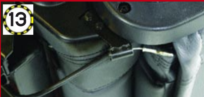
13 Take the wire for the tilt connection, which was removed in step 8, and feed it through to where it should be fitted. Use a pair of pliers to hook it into position
