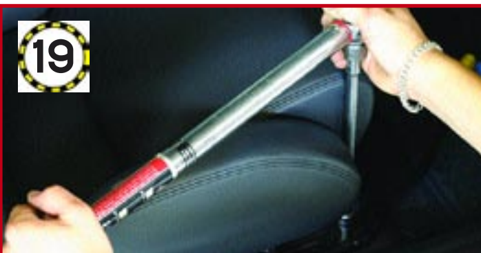
19 When you've fitted all four Torx bolts for the runners, use a torque wrench to fully tighten them to 35Nm
