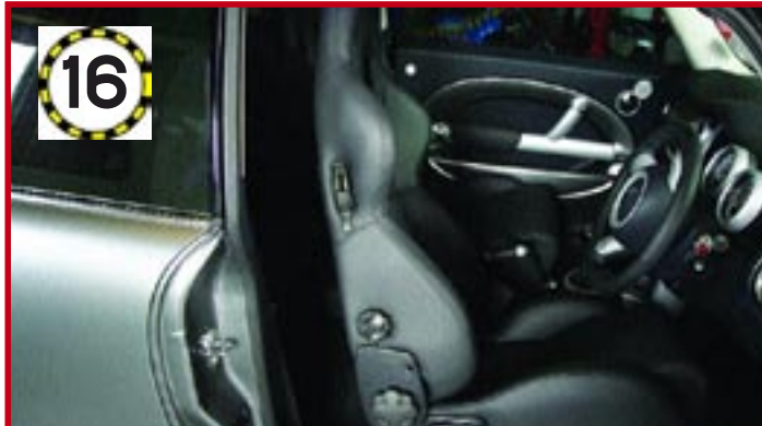
16 To fit the new seat into the car, move it fully forward on its runners and tilt it forward if necessary. Lower it gently into the car. Make sure the runners don't catch the paintwork
