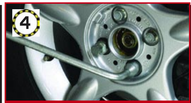
4 Slacken all four wheel bolts. Don't fully loosen or remove them yet. Use the key for the locking wheel nut
