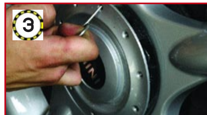
3 If your wheels have a hubcap fitted, lever it off with the key provided in the standard toolkit
