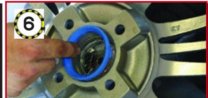
6 Some aftermarket wheels are supplied with a plastic locator to help fit them onto the hubs. Fit the locators if they are supplied
