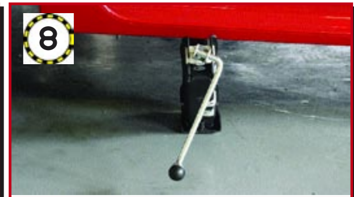
8 When removing a rear wheel, place a chock under the front of the adjacent front wheel and raise the car on the rear jacking point. After fitting all the wheels, recheck the nuts
