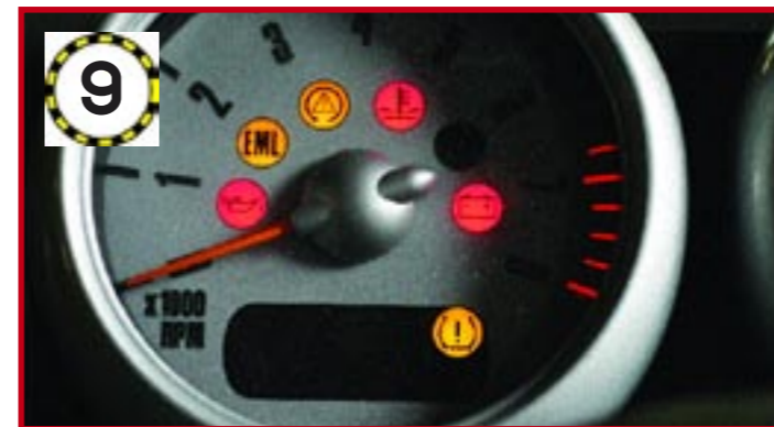
9 If you've changed to larger or smaller sized wheels and tyres, the runflat sensor light may light up when the ignition is switched on. If it stays on, the sensor has detected a change in the wheel/tyre diameter. See the next step to fix this
