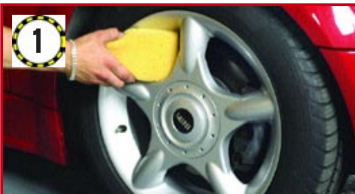
1 Place the car on a flat surface. Pull the handbrake on and select first gear. Wash all the wheels to remove any harmful road dirt or brake dust
