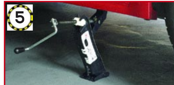
5 Use the jack found in the toolkit and place it under the front jacking point. Raise the car enough to remove the wheel and undo the wheel nut
