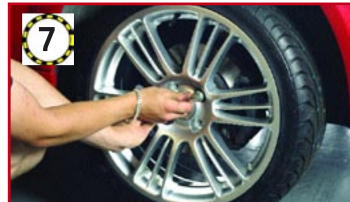
7 After removing the original wheel, fit the new wheel, tighten the bolts, then lower the car to the ground and fully tighten them to 110Nm
