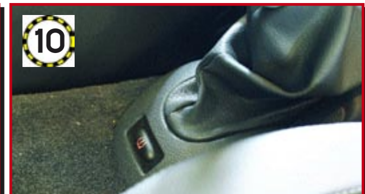
10 If the run flat sensor remains illuminated, it will need resetting. Switch off the ignition, press and hold down the button for the sensor (below the handbrake), switch on the ignition and wait for a beep. Release the button, then switch the ignition off then on again
