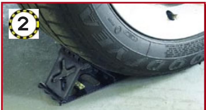
2 To remove the front wheels, place a chock under the rear of the rear wheel, which is on the same side of the car as the wheel you want to remove
